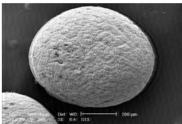
Figure 1: SEM Images of Ferric Saccharate Microcapsules Prepared by Extrusion Method Through Needle
